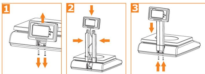
**Tower is included** in the scale box (except "Weight Only" models) and can be easily set up by the user.
